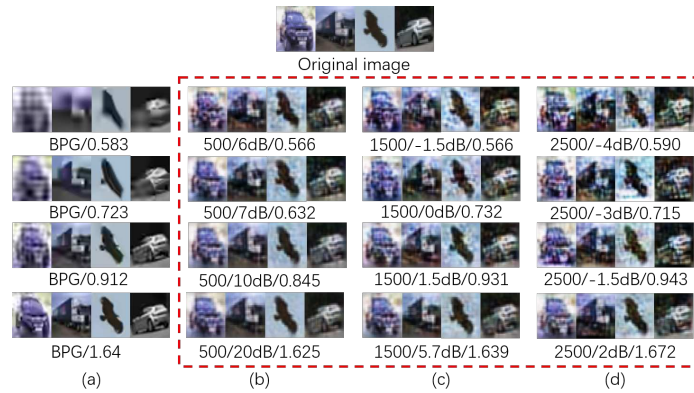
Fig. 8. Visual comparison of reconstructed images from C-JSCC and BPG at different bpp (columns (b-d) are outputs of C-JSCC, \text{SNR}_{\text{train}}=20\text{dB} , \lambda = \tau = 0.01 ), the text below each image indicate parameters K/\text{SNR}_{\text{test}}/\text{bpp} .
